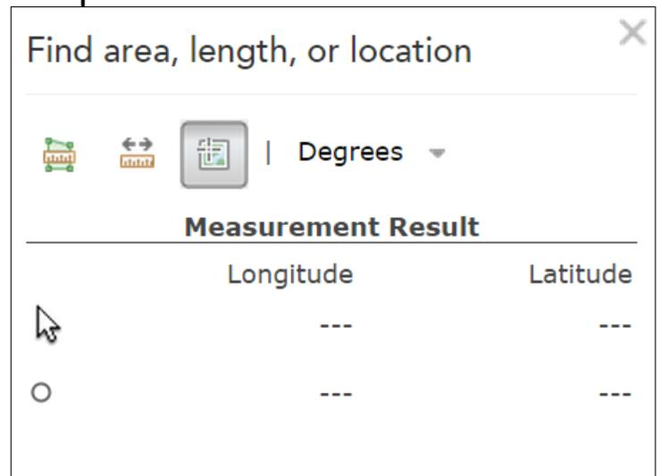
The location tool stores coordinates for one location at a time with stored values displayed on the lower line with the hollow point. The tool continues to retrieve coordinates for the places you scroll over with the mouse cursor on the viewer screen and these values are displayed on the top line of results.
