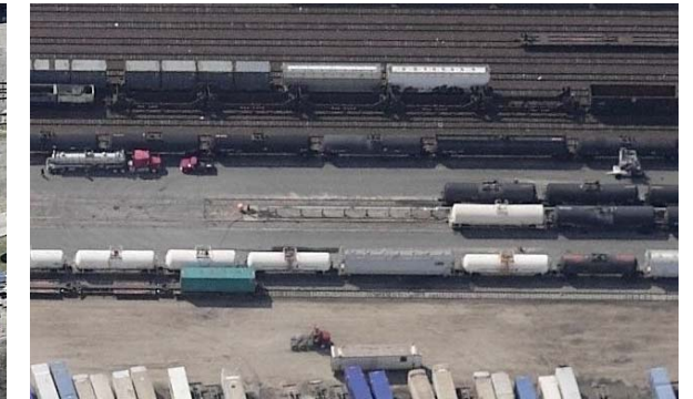
Figure 3-10 A Liquid Bulk Transfer Facility with Direct Truck Access to Railcars
