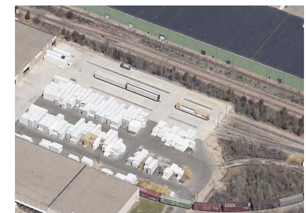
Figure 3-6 Centerbeam Flats at a Building Materials Transload Facility
