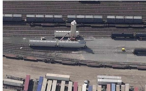
Figure 3-8 Dry Bulk Transfer to Intermediate Silo
