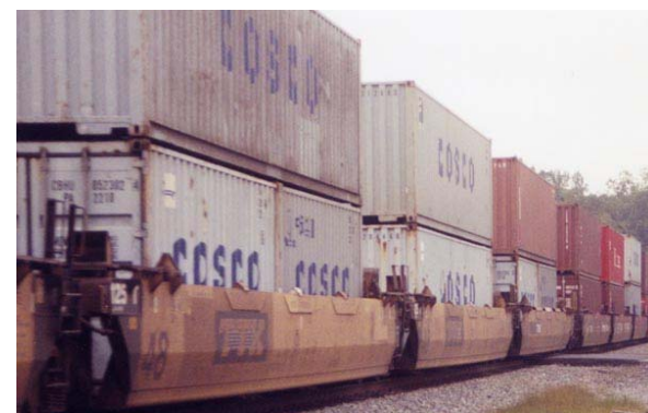
Figure 3-2 Double Stacked International Containers in Well Cars
