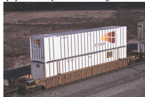
Figure 3-1 Double Stacked Domestic Containers in Well Car
