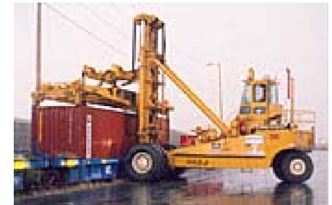
Figure 3-4 Side Loader Lowering a Container into a Well Car
