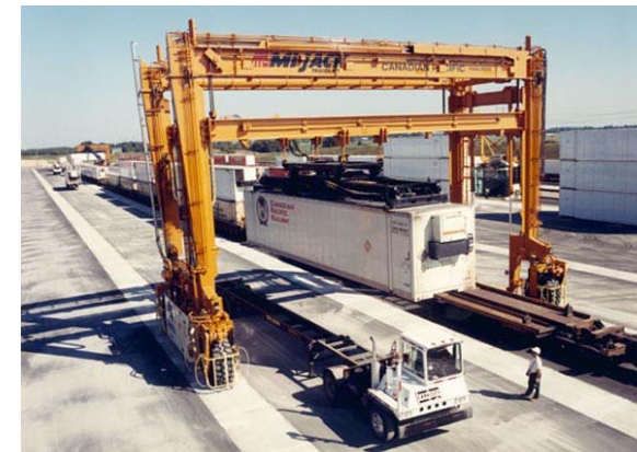
Figure 3-3 Rubber Tired Gantry Crane Loading a Container on to a Chassis
