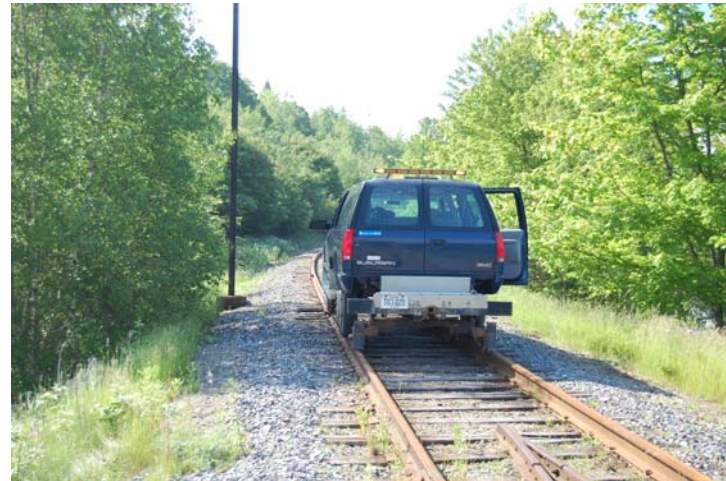
Figure 5-1 Hi-Rail Vehicle on Pan Am Track
